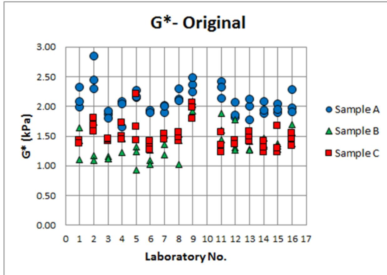
Figure 6-1. variation of the complex modulus  $G^*$  for the three replicates tested by the 15 laboratories for the three samples A, B, and C.
