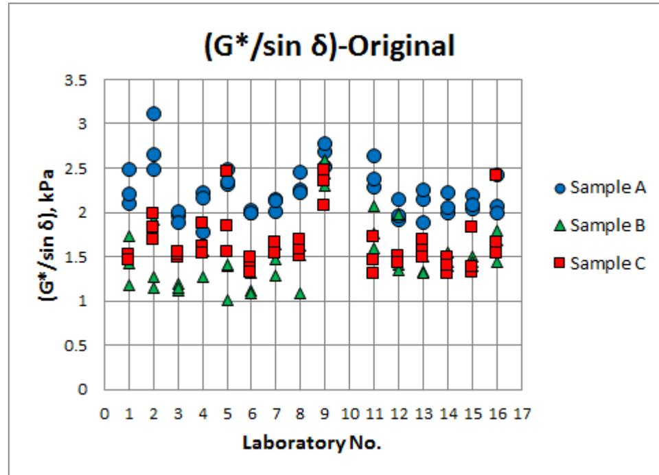
. Example scatter plot of test results ( $G^*/\sin\delta$ ) of the three samples (3 replicates per test)
