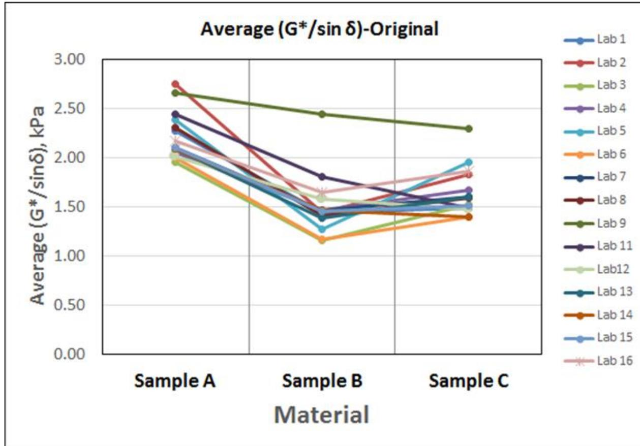
Figure 3-6. A plot of the average  $(G^*/\sin \delta)$  for the three original (unaged) binders as tested by all laboratories in the current ILS. The plot is used to detect interactions.
