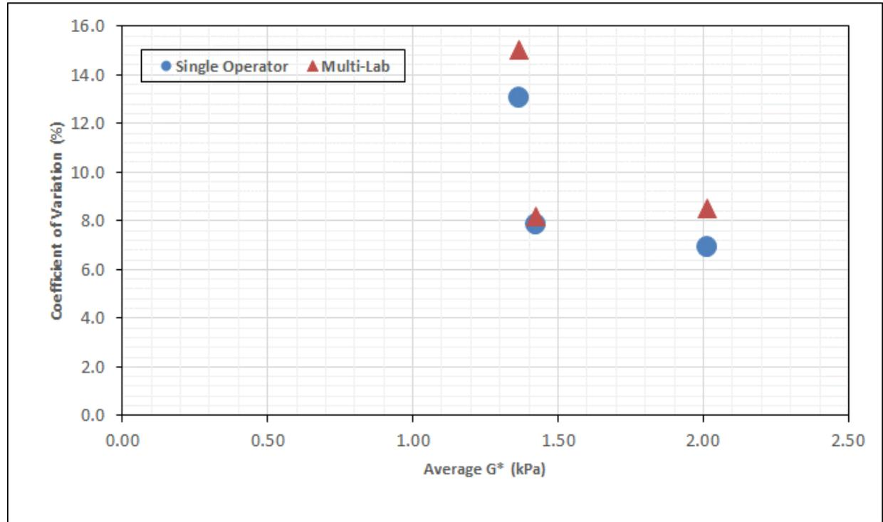
**Figure 6-5. Variation of the single-operator and multilaboratory standard deviation and coefficient of variation with average  $G^*$ -Original.**
