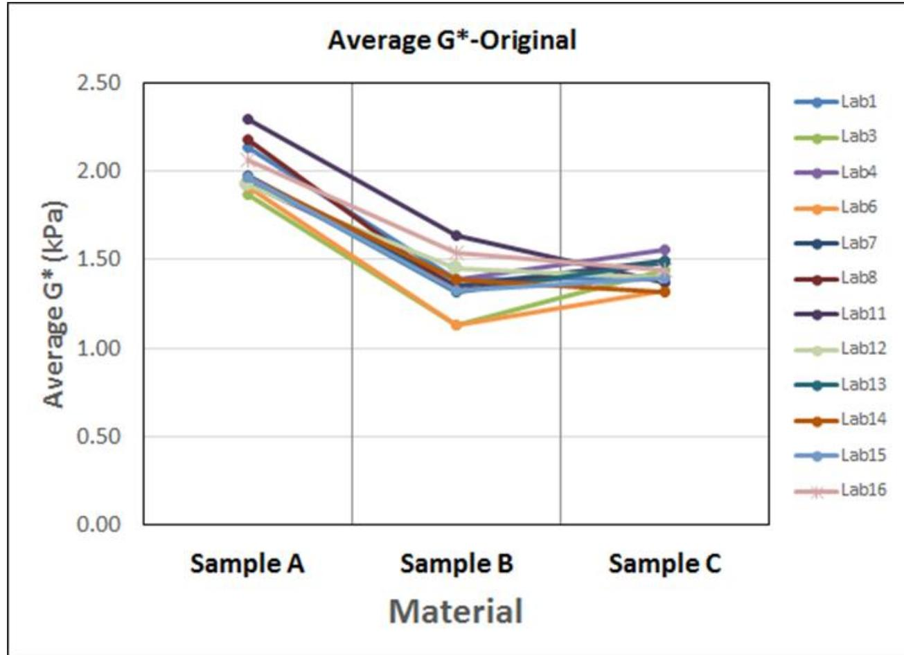
Figure 6-4. Variation of average G\* per material type for the 12 labs used in subsequent precision analysis.
