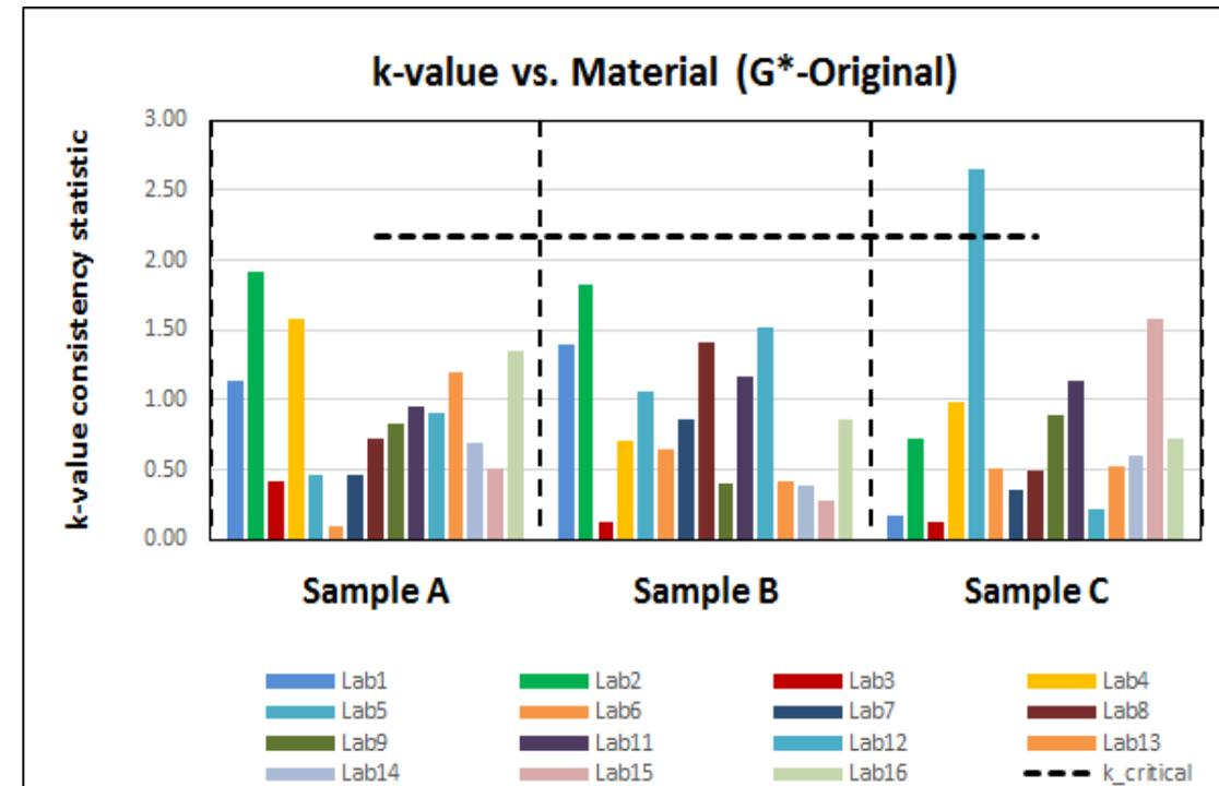
Figure 6-3. The consistency h-value and k-value plots for G\*-original plotted by material type.
