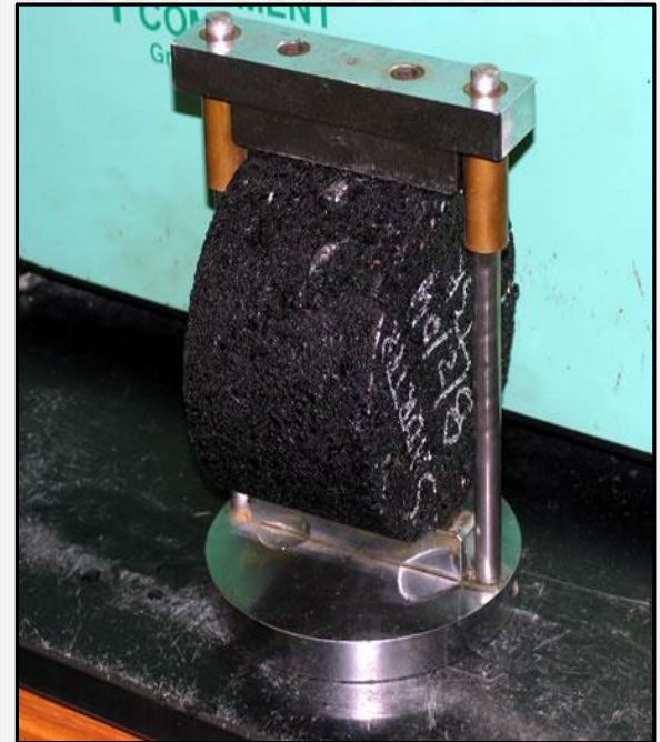
Foamed Asphalt ITS @ 77 Deg. F.
